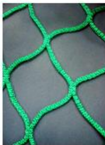
Fig. 3: Net made with double bar raschel machine
